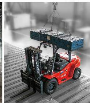
Impact test of overhead guard
