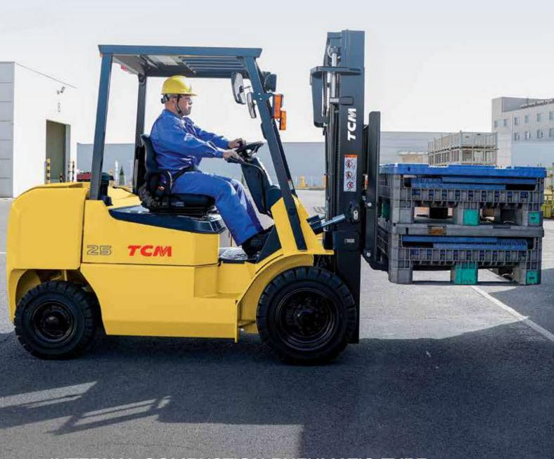
INTERNAL COMBUSTION PNEUMATIC TYRE FORKLIFT TRUCK
